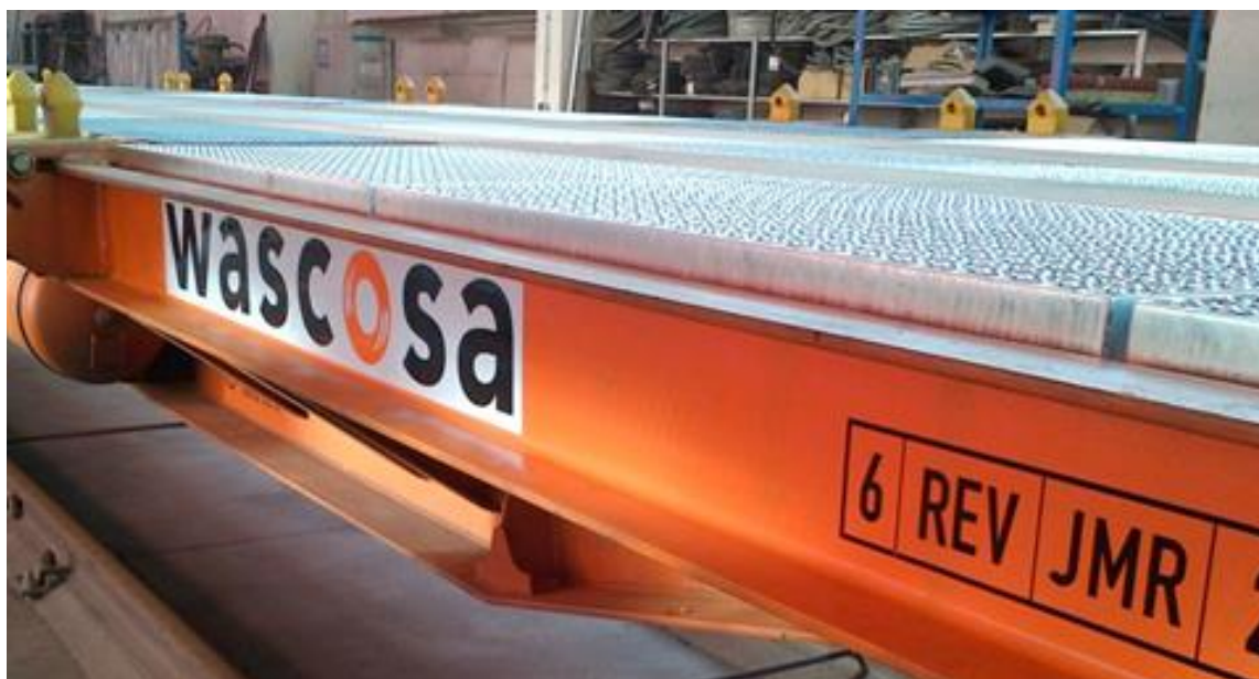
Figure 4: Wascosa container wagon with accessible floor
