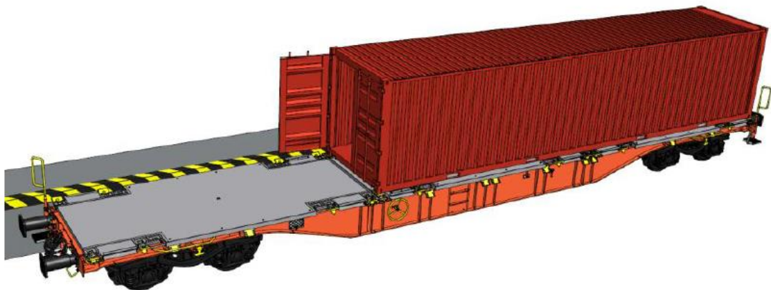
Figure 7: 60ft platform solution – 3D drawing
