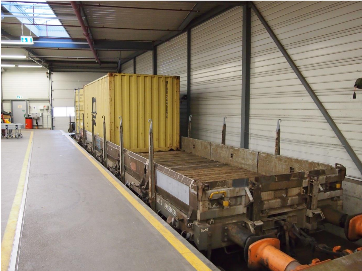
Figure 1: Current wooden floor wagon for container transports into sidings
