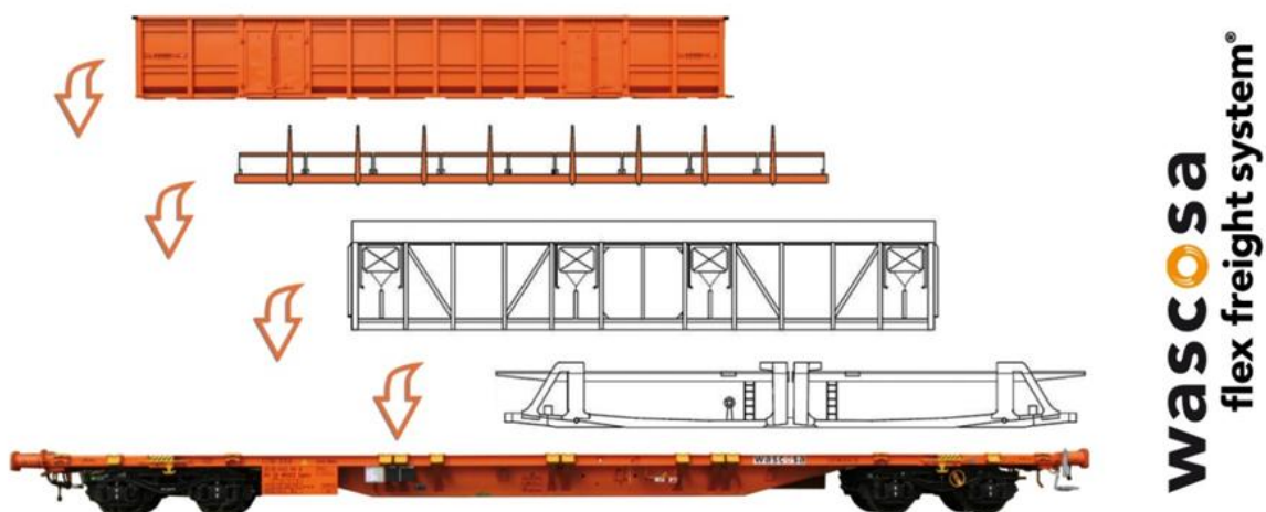
Figure 1: General concept of Wascosa flex freight system ®
