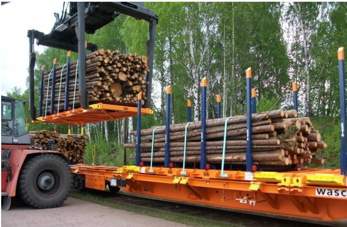
Figure 2: Non stackable timber cassettes on Wascosa flex freight system ®
