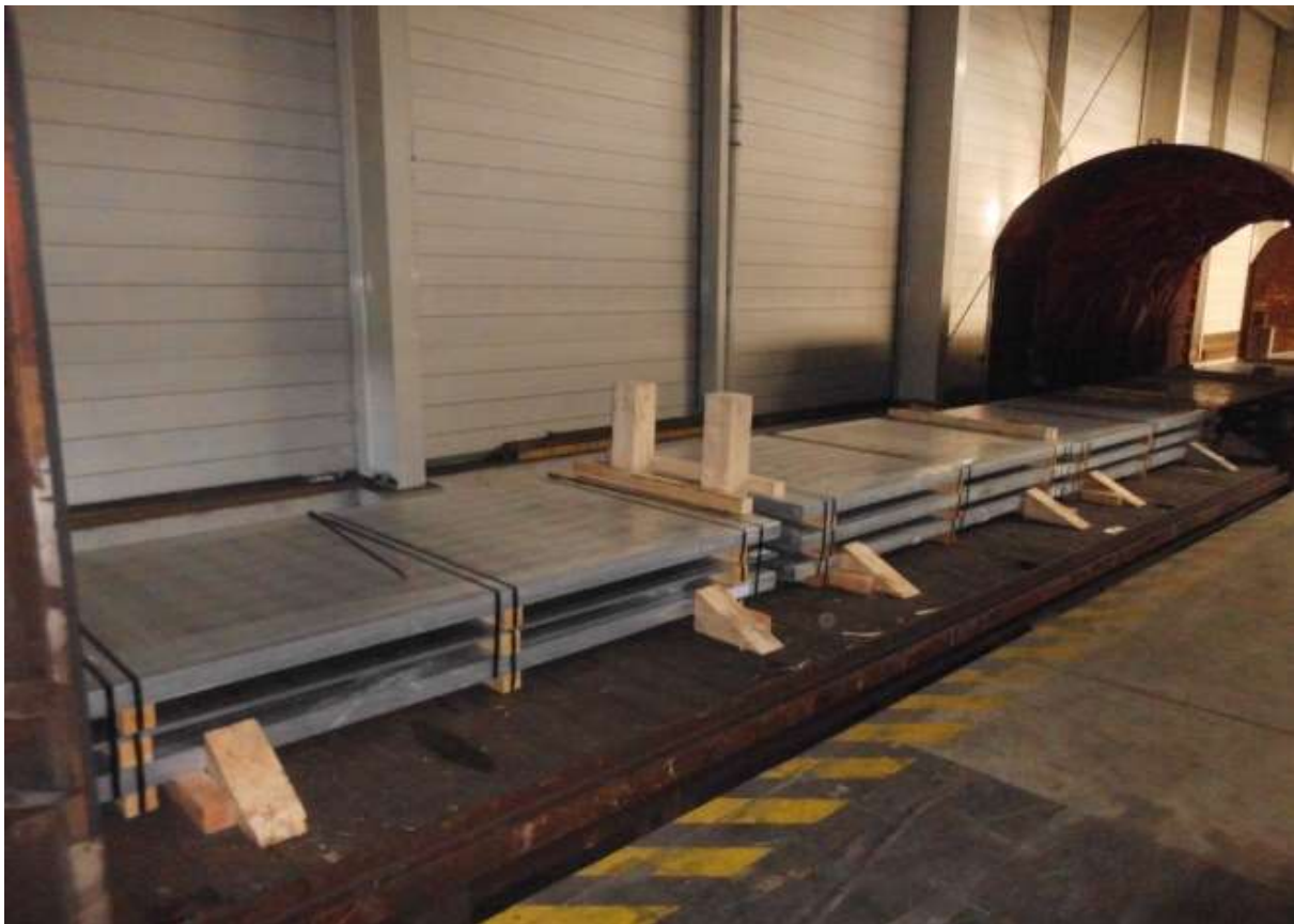
Figure 3: Steel plate bundles on rail wagon in the RLC Nordhorn
