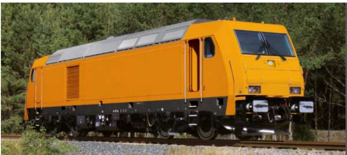
Figure 2: Locomotive type Bombardier TRAXX F140 DE
