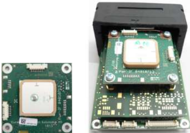
Figure 11: WPAN radio communication PCB
