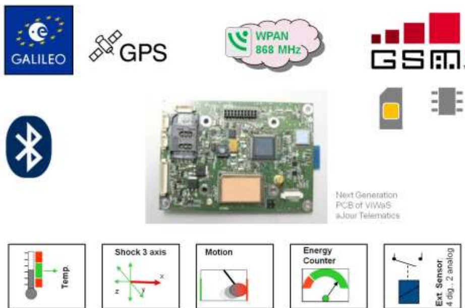
Figure 8: Functionality of new ViWaS telematics
