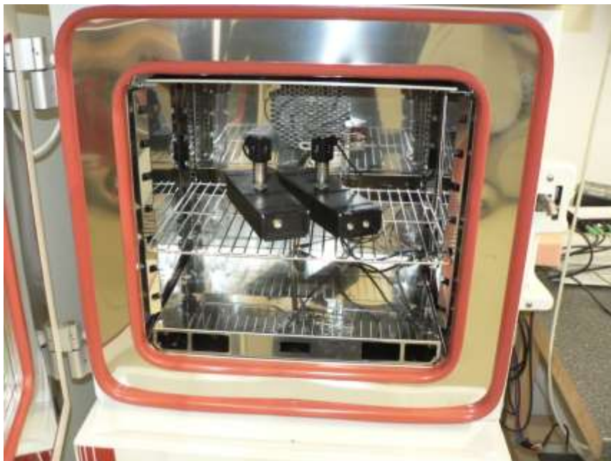
Figure 6: Housings with pressure transducer in the climate chamber.
