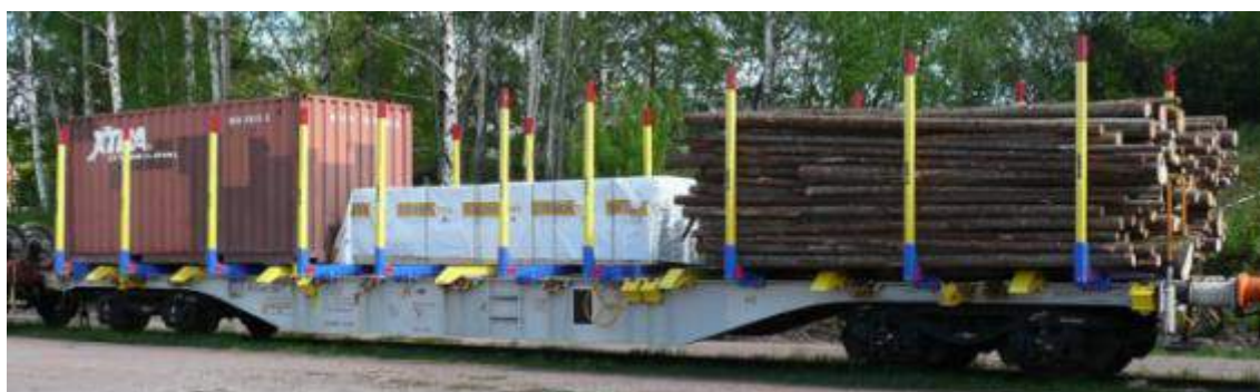
Figure 37: Ahaus Alstätter Eisenbahn Sgns container wagon for multiple commodities: containers, packaged lumber and logs.
