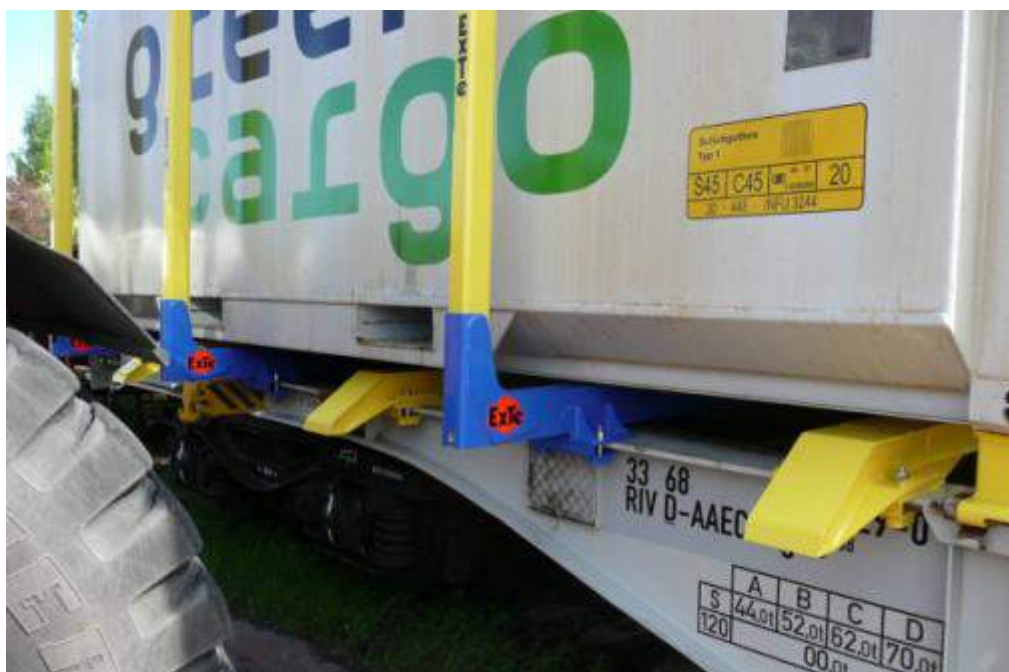
Figure 39: Installation of ExTe SR 8 log bunks and cross beams on Ahaus Alstätter Eisenbahn Sgns container wagon
