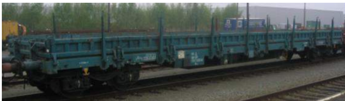
Figure 33: B-Cargo Res/Regs wagon for containers and multiple commodities such as steel shapes and plates
