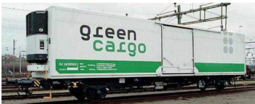
Figure 41: Insulated superstructure “Maxi-Låda” with cooling unit fitted onto Lgjs container wagon
