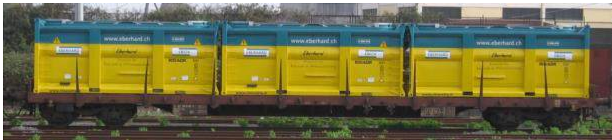
Figure 34: FS Rgs wagon for containers and multiple commodities such as steel shapes and plates
