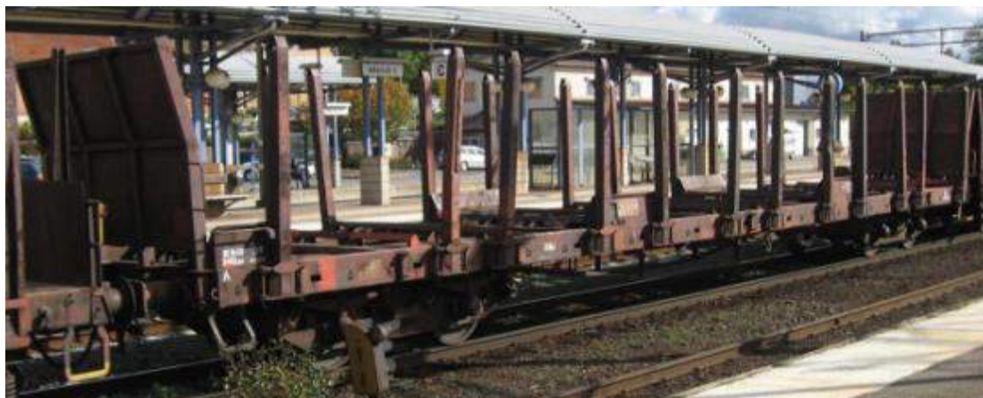
Figure 35: Green Cargo Sgs wagon designed for dual commodities: containers and logs
