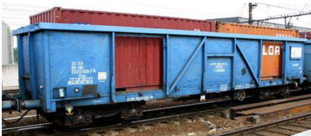
Figure 31: Inter Ferry Boats/B-Cargo Eaos gondola loaded with containers
