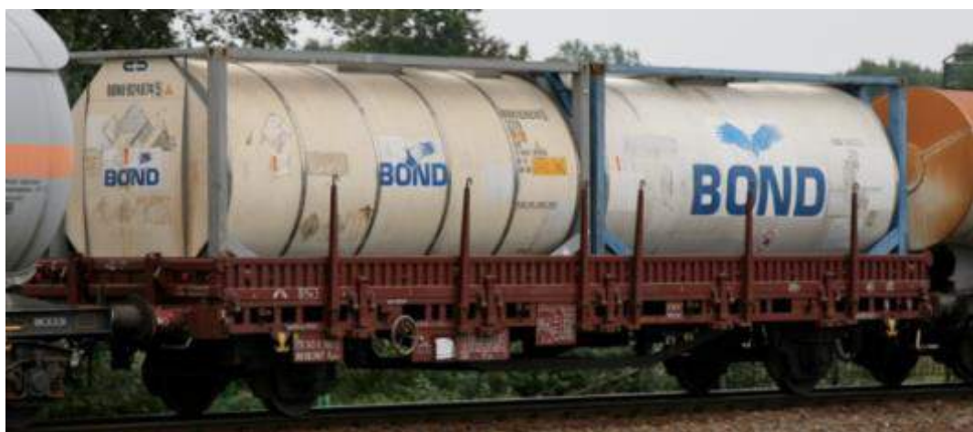
Figure 32: PKP Cargo Kgn's wagon with folding sides, side stakes and container pedestals for multiple commodities
