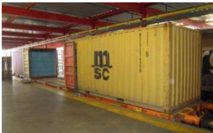
Figure 8: Test of 'Flex Freight Car' with iron grid inlay at Migros siding in Neuendorf (CH)
