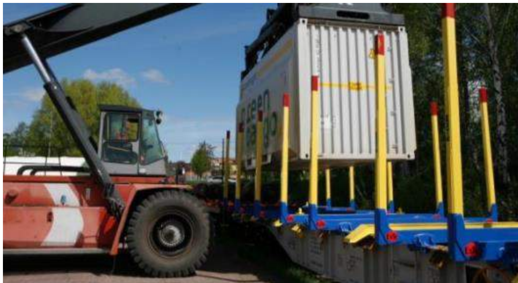
Figure 38: Loading of woodchip container onto Ahaus Alstätter Eisenbahn Sgns container wagon with ExTe SR 8 log bunks
