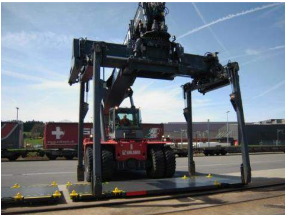
Figure 12: 20' 'Container Loading Adapter', handling by reach stacker
