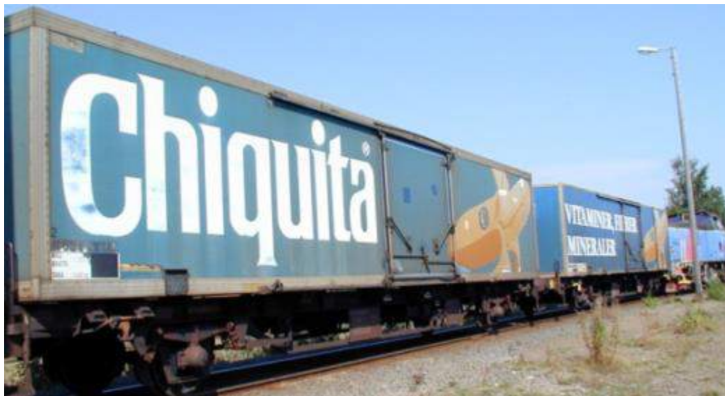
Figure 40: Insulated superstructure “Maxi-Låda”. Fitted onto Lgjs container wagon
