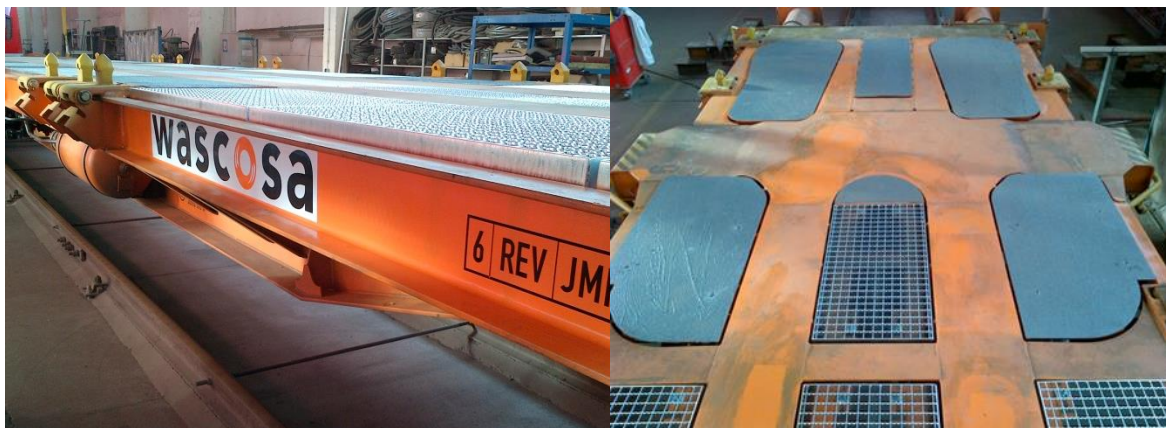
Figure 8: Wascosa 'Flex Freight Car' with iron grid inlays
