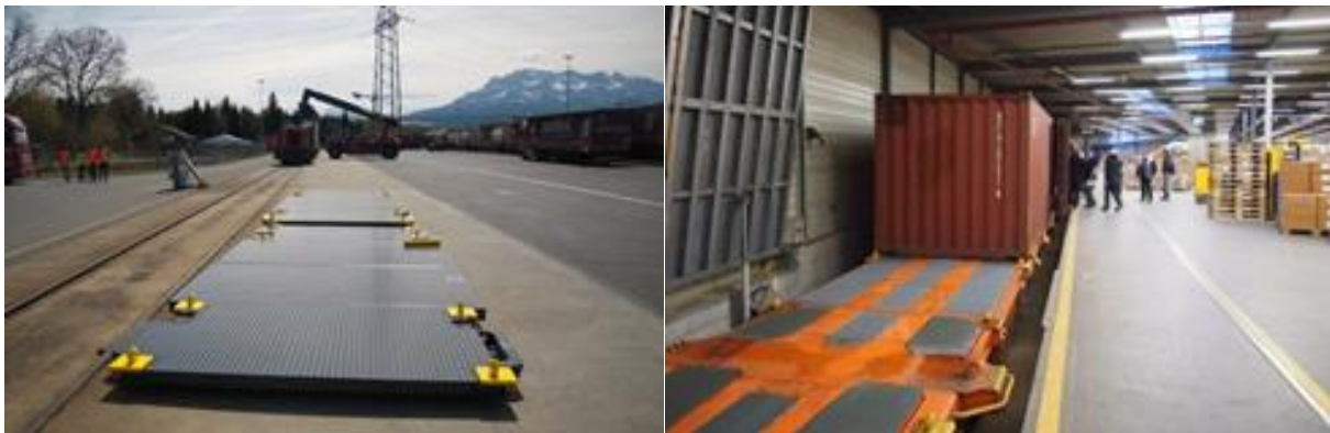
Figure 3: Wagon equipment for container loading and unloading in sidings
